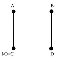
Figure 1: A simple rectangular warehouse with two (vertical) aisles and four pick locations. Dimensions are such that picking e.g. an SKU from location B takes a travel distance of 4.
